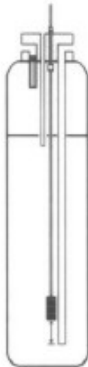
DIAGRAM 4 – DOUBLE AERATION ASSEMBLY
